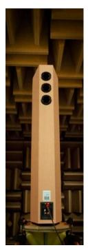
Our speaker design and manufacturing facility in Canada has a very unique advantage – an on-site 'anechoic chamber'. Anechoic chambers are reflection free rooms and are used by the superior speaker manufactures to do all the loudspeaker testing in an environment where early reflections and outside noise issues are eliminated from the measurement curve(s). Anechoic cambers are very, very expensive to build but they are invaluable when designing a quality loudspeaker.
